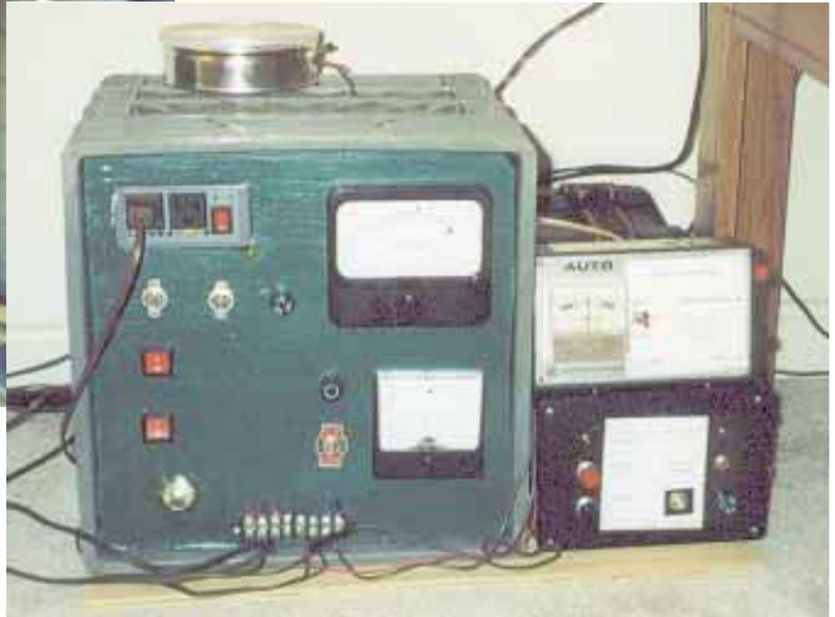
Right: A homemade power center with metering, fuses and disconnects, charge regulator, and low voltage disconnect.
