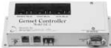
The optional GC-1 GenSet Controller provides fully automatic power management by automatically starting and stopping your generator when your battery(s) are discharged and recharged to user selectable levels.
